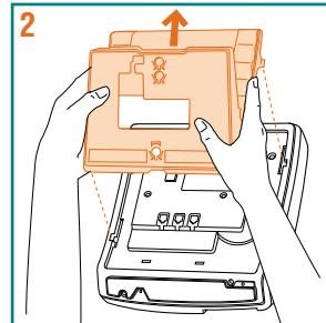
Lift the stand out of the slots on the base.
